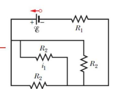
(a) The parallel set of three identical  $R_2 = 18 \Omega$  resistors reduce to  $R = 6.0 \Omega$ , which is now in series with the  $R_1 = 6.0 \Omega$  resistor at the top right, so that the total resistive load across the battery is  $R' = R_1 + R = 12 \Omega$ . Thus, the current through R' is (12V)/R' = 1.0 A, which is the current through R. By symmetry, we see one-third of that passes through any one of those 18  $\Omega$  resistors; therefore,  $I_1 = 0.333 A$ .
